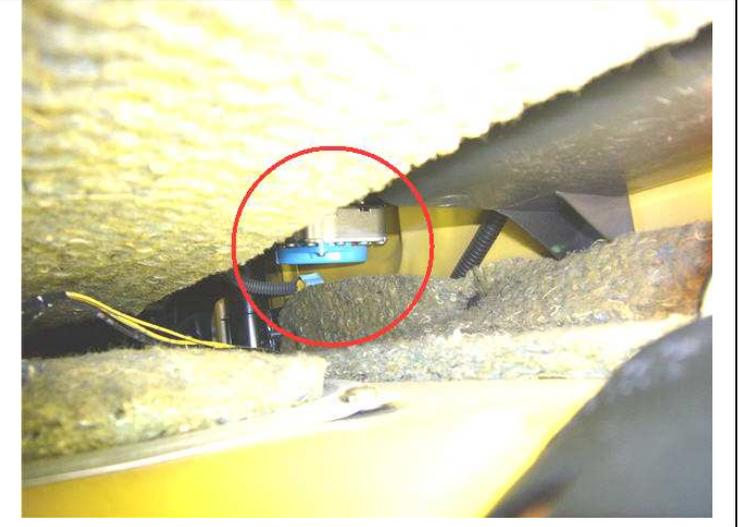
Take a minute to review the next few photos to get a feel for how the SBL mounts to the seat belt assembly. The seat belt assembly has a large square nut on the right side of the bracket and the SBL is designed to fit over the nut. Because you cannot directly see the nut you will have to place the SBL over the nut by feel. Fortunately this not very hard to do and shouldn't take more than a minute or two once you get in position.
