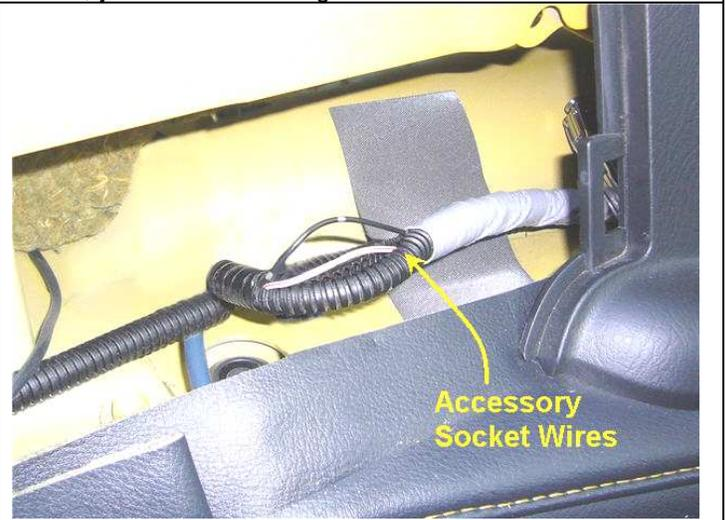
**4. Attach T-taps** to the Accessory Socket wires. Make sure the wire is positioned in the groove of the metal part of the T-tap and close the pliers until the locking tab snaps closed. Here's a photo using regular pliers (opened up to the wide-jaw position) to clamp the T-taps. Note – you are connecting to the **black** and **white/red** wires, this blue is just a demo.
