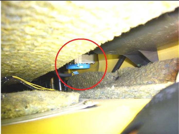
Take a minute to review the next few photos to get a feel for how the SBL mounts to the seat belt assembly. The seat belt assembly has a large square nut on the right side of the bracket and the SBL is designed to fit over the nut. Because you cannot directly see the nut you will have to place the SBL over the nut by feel. Fortunately this not very hard to do and shouldn't take more than a minute or two once you get in position.
