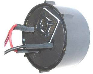
**Wiring** – Only 3 connections to the car are needed: +12v, ground, and a tachometer signal
