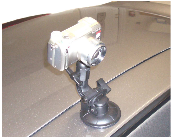
Photo 4 – Install your camera – tighten lock ring against bottom of camera to be sure camera doesn't come loose.
