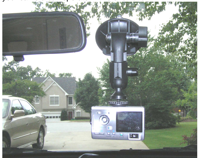
Photo 6 – Upside down mounting on windshield – only if your camera can operate in this orientation.
