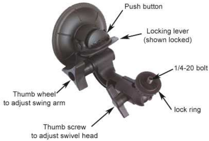
Photo 1 – Camera Mount parts
