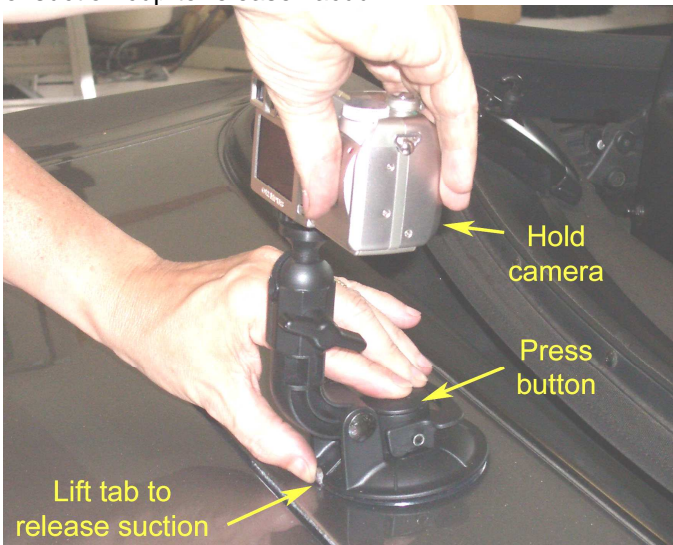
Photo 5 – Remove by pressing button and lifting tab on edge of suction cup to release vacuum.
