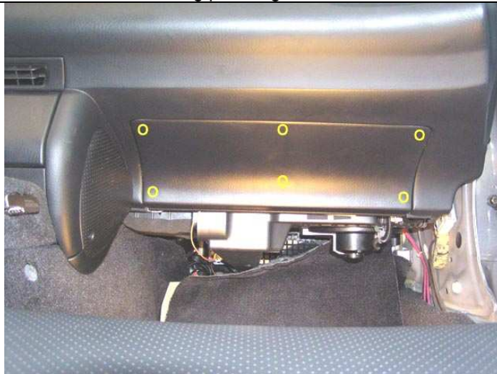
Photo 1 showing passenger dash access cover
