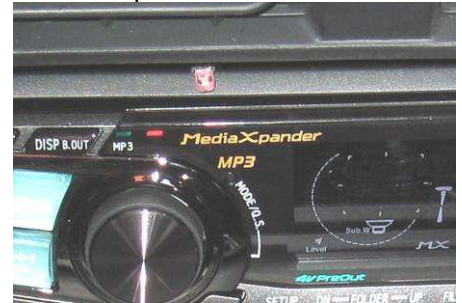
Close-up of IR emitter above HU
