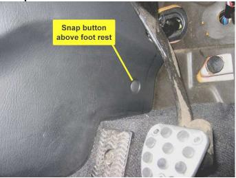
Photo 5 – Remove snap that gets stuck in foot Photo 6 – Replace snap in foot well trim panel well wall
