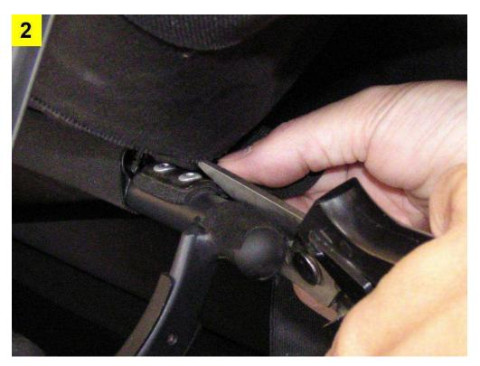
**3. Hold the Modifry strap like this.** Make sure the pins are facing you, and the pin closest to the edge of the strap is towards the center of the car. You will insert this pin into the inboard rivet hole. The pins are glued into the strap and should not fall out with normal handling.
