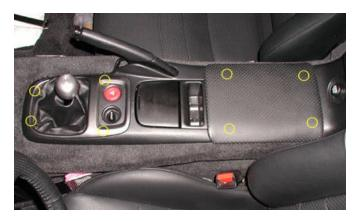
Tilt up the rear of the cover and unplug the ROOF and HAZARD switch connectors, shown here.
