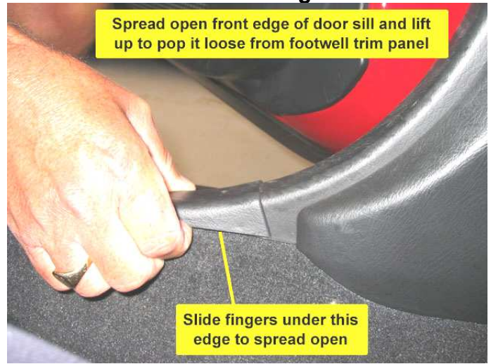
Photo 2 – Lift front edge of door sill
