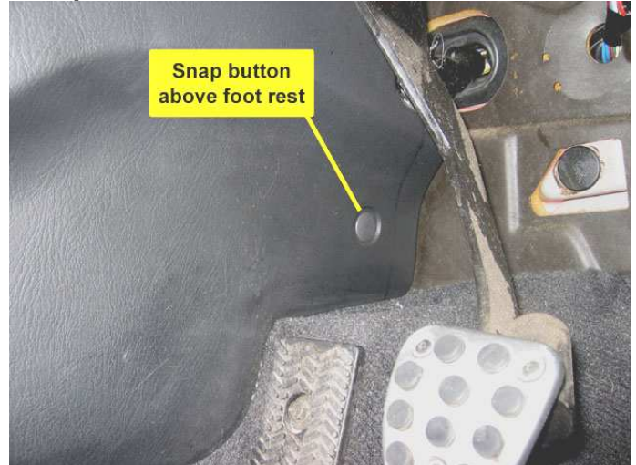
Photo 4 – Remove inside snap on foot well trim panel
