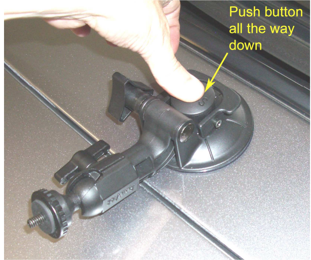
Photo 2 – Press button firmly to release air
