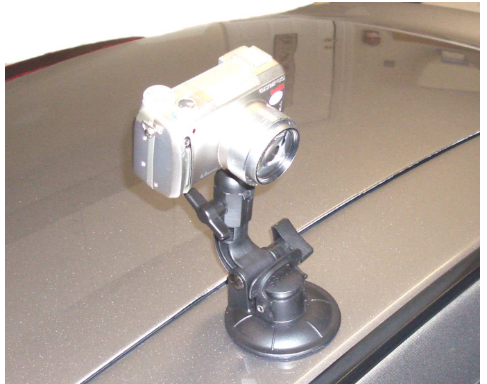
Photo 4 – Install your camera – tighten lock ring against bottom of camera to be sure camera doesn't come loose.
