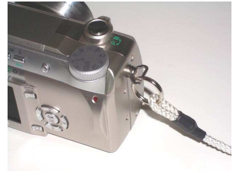
Photo 6 – Attach tether to camera
