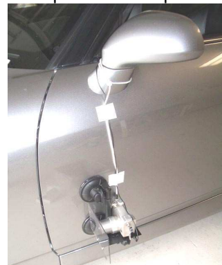
Photo 8 – Tether tied off to mirror and microphone wire taped down
