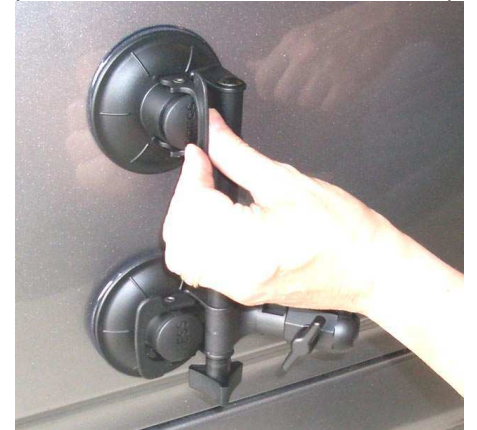
Photo 2 – Lift locking lever, then repeat photos 1 and 2 for bottom suction cup
