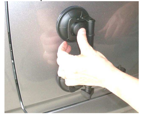
Photo 2 – Lift locking lever, then repeat photos 1 and 2 for bottom suction cup
