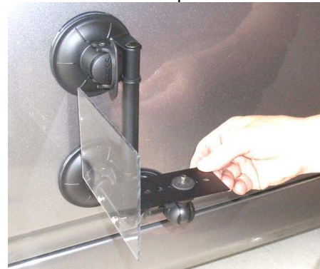
Photo 8 – Tether tied off to mirror and microphone wire taped down
