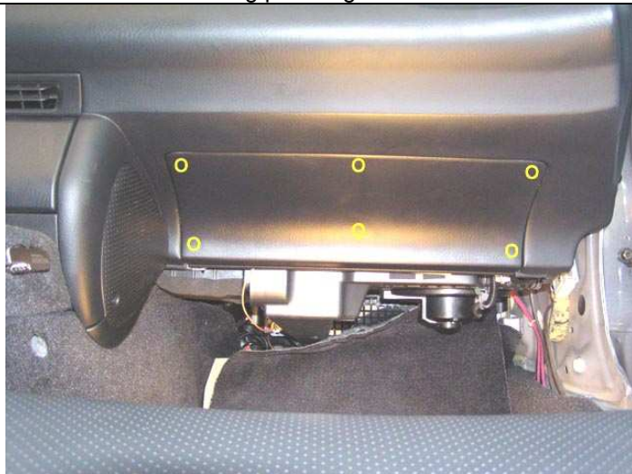
Photo 1 showing passenger dash access cover
