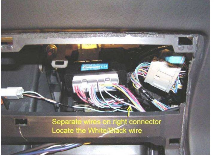
Photo 2 – Convertible Top Module and Speed Signal Wire
