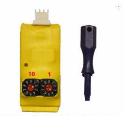
Left switch is the 10's digit, right switch is 1's This module is set to "24" for a correction of 12%
