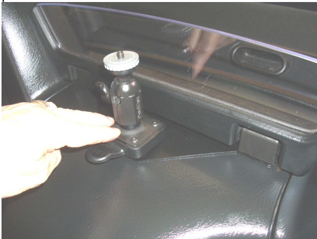
Photo 5 – Press on front edge of pedestal to lock it into position. Lift lever to remove.
